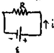
Writing loop equation:  $\mathcal{E} - iR = 0 \Rightarrow i = \frac{\mathcal{E}}{R} = \frac{4 \text{ V}}{10 \Omega} = .4 \text{ A}$ , counterclockwise.
