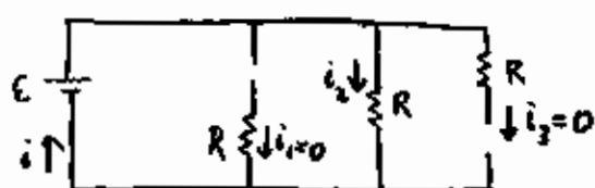
Since  $i_1 = i_3 = 0$ ,  $i = i_1$ , where  $i$  is the current thru the switch. Writing a loop equation:  $\epsilon - i_2 R = 0$
