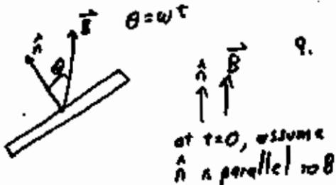
9. A circular coil of 10 turns and area  $6 \text{ cm}^2$  rotates with an angular velocity of  $2\pi \cdot 60$  radians per second around an axis perpendicular to the uniform  $B$  field.  $B = 0.2 \text{ T}$ . The axis of rotation goes through a diameter of the circular cross section of the coil. What is the emf  $|E|$  when  $\theta = \frac{\pi}{3}$  as shown above?
