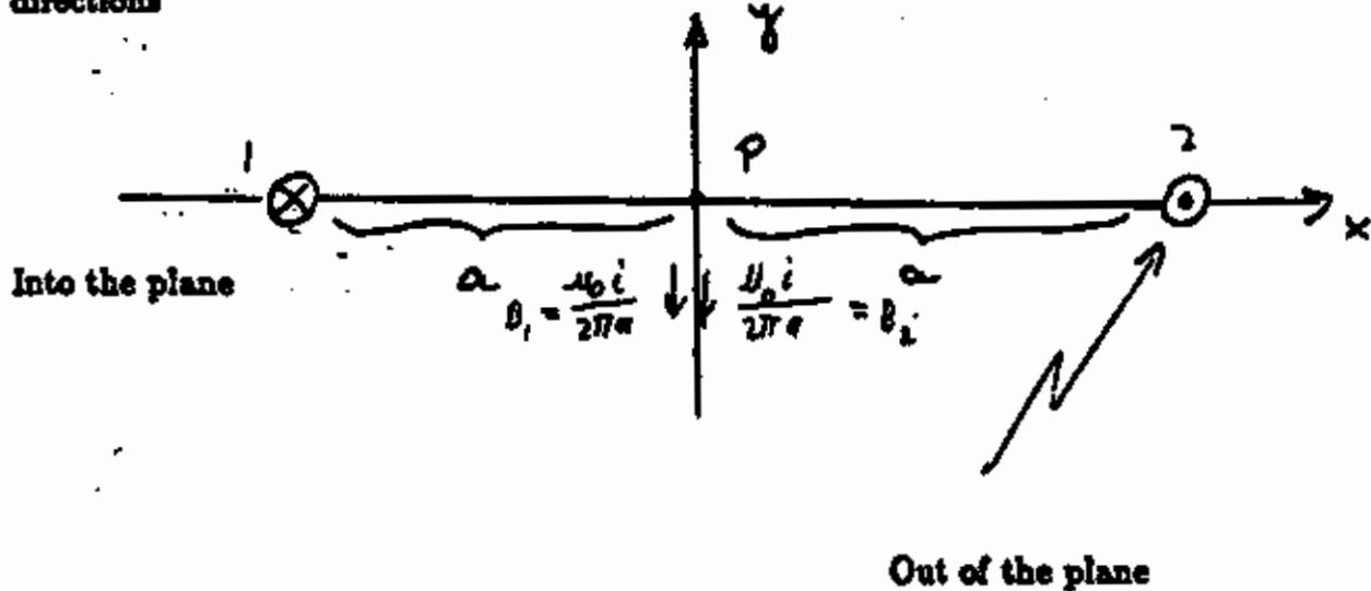
$a = 0.32 \text{ m}$ . What is the magnitude and direction of the resultant  $\vec{B}$  field at the midpoint  $P$ ?
