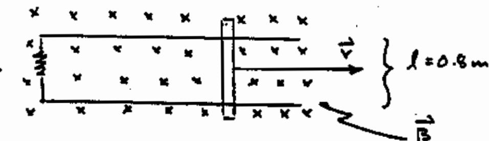
A uniform  $B$  field is perpendicular to the plane of the rails and goes into the plane of the paper.  $P = i^2 R = 2W$  is dissipated in  $R$  when the rail is pulled at constant velocity  $v = 3 \text{ m/sec}$ . What is the value of the  $B$  field?
