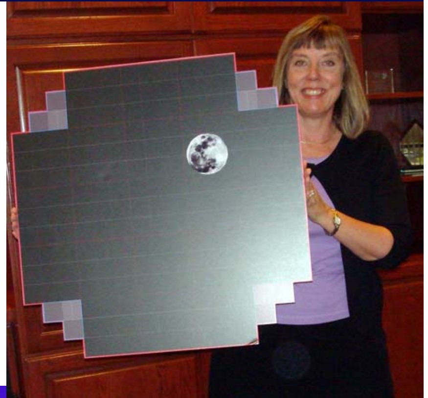
Figure 2.9: With its 189 sensors, each a 4K x 4K charge-coupled device (CCD), the focal plane of the camera images 9.6 \text{ deg}^2 of the sky per exposure. Note the presence of wavefront sensors, which are fed back to the mirror support/focus system, and the guide sensors, to keep the telescope accurately tracking on a given field.
