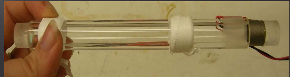
The Fabry-Perot Interferometer Cavity
